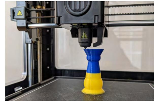
Z-Pause can also be used to add material to the inside of an ongoing print. One reason we might do this is to add magnets or even enclosing a bearing on the print like we did above. This technique is great for making musical instruments (by adding beads), making magnets, securing items in place, and even as shock absorbers (by adding hot glue to the inside of the print).
