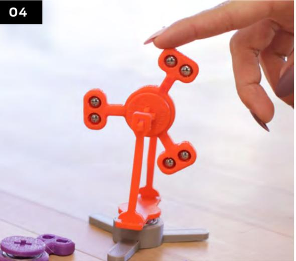
One partner will hold the rotor in place with one hand and apply a consistent rotational force on the fidget spinner each time. Immediately after spinning the fidget spinner in place, release the rotor being careful to avoid applying a sideways force.
