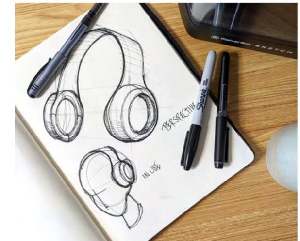
**Three-point Perspective:** A sketch drawn in a three-point perspective is similar to the image one sees when looking into a horizon and seeing a road converge into a singular point. These sketches tend to be more powerful because it is able to show multiple sides of a proposed idea from one sketch alone.
